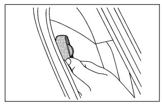
1. Pull the elastic cord out from between the edge of the seatback and the interior body to remove the guide from its storage clip.
